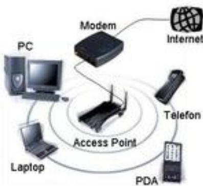
Figure 1: A number of devices are connected with each other via the access point and with the Internet via the modem.
