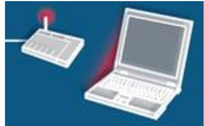
The data that need to be sent from one device to another are transmitted using a high-frequency radio link instead of a cable. Devices connected to a WLAN can both receive and transmit.
